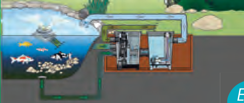
Schematic diagram: ProfiClear Premium Compact gravity-fed
