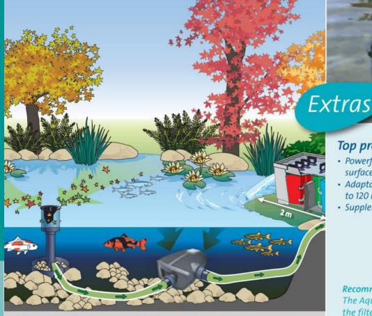
Schematic diagram: AquaSkim in use with filter and watercourse pump AquaMax Eco Premium
