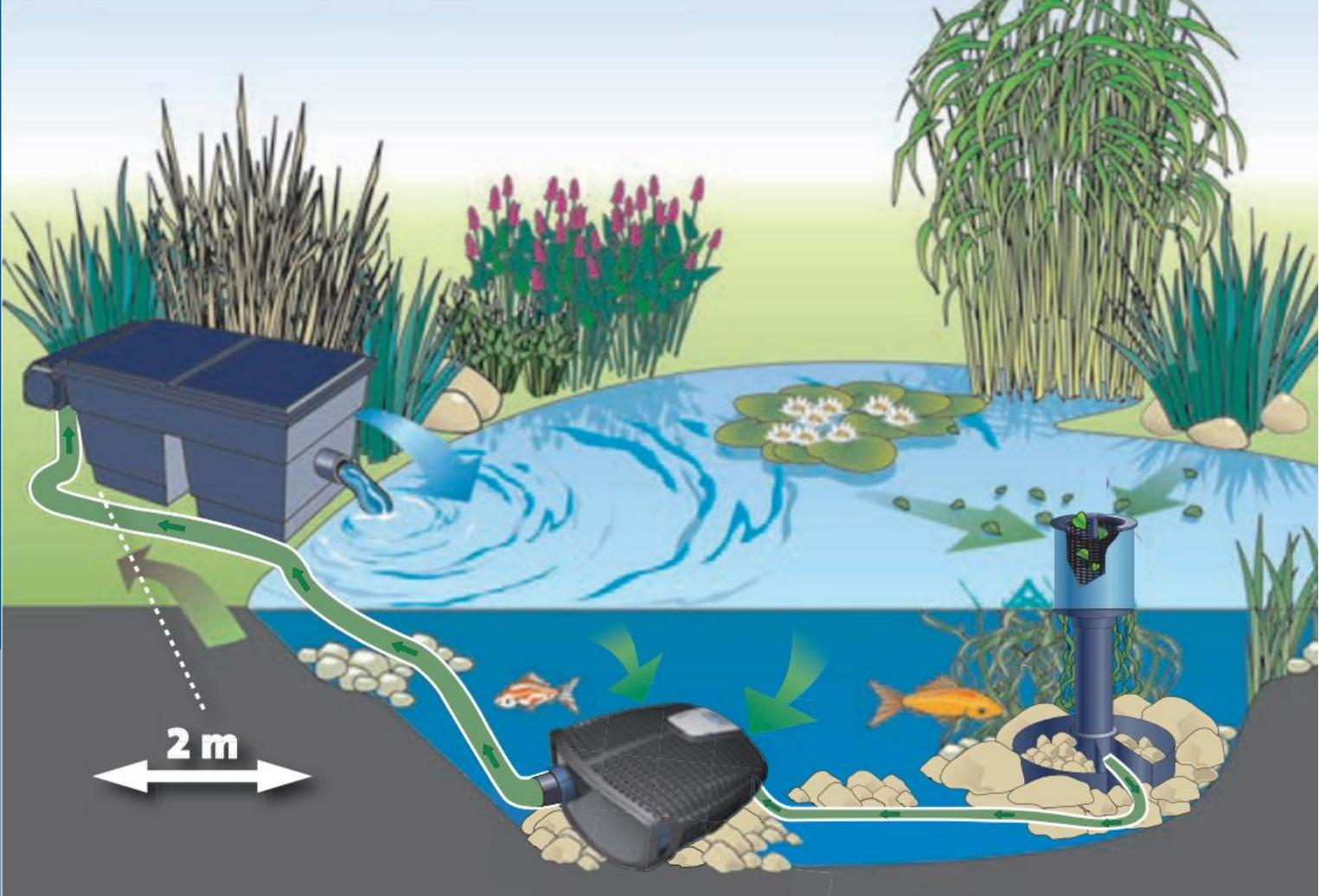
Schematic diagram: Filter and watercourse pump AquaMax Eco Twin with an OASE flow through filter and additionally connected OASE skimmer AquaSkim 40
