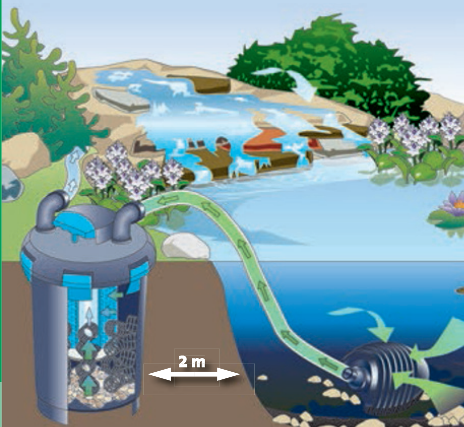
Schematic diagram: Pressure filter in combination with filter and watercourse pump
