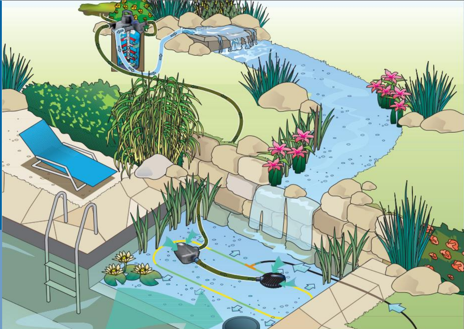
Schematic diagram: Filter and watercourse pump AquaMax Eco Premium 12 V used in the swim pond in combination with an OASE pressure filter FiltoClear
