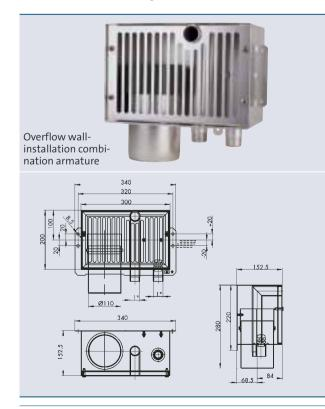
the muff of the channel pipe. The fresh water feed pipe and the connection of the cable protection pipe for the water level sensor are connected to the appropriate threaded nipple via PE pipe unions. The overflow funnel can be pushed up or pushed down 20 mm to adjust to the water level.
